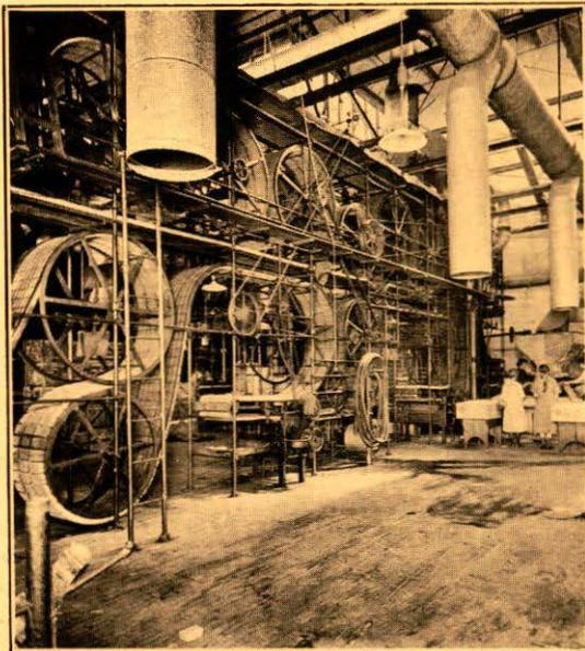
*Drying the Matches on Endless Chains*
