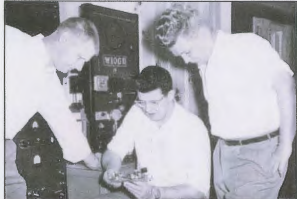
Al Hankinson, Dick Wright and Gus Fallgren compare their mite-sized transmitter with standard transmitter in background. Drastic reduction in size was achieved by using two Raytheon transistors.
