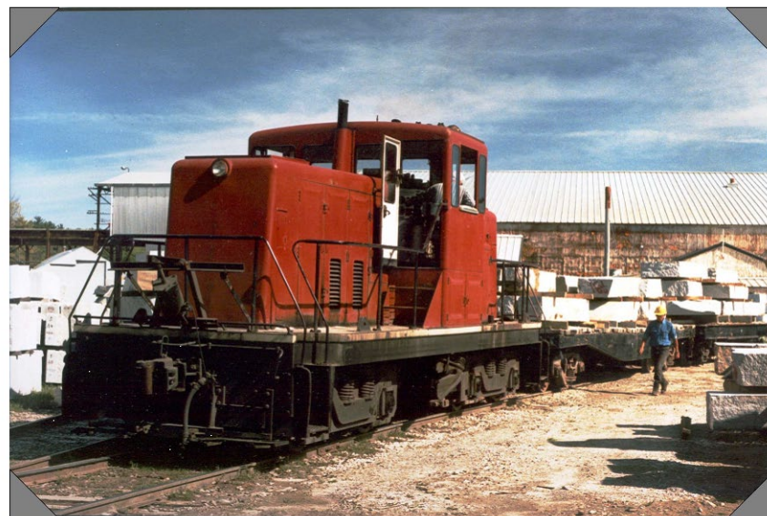
Granite being moved from the quarry to the cutting shed on the south side of Route 40 (Groton Rd.). The 80-ton G.E. diesel electric locomotive was purchased in July 1953 and is nicknamed “The Locy” by Fletcher employees. (A Fletcher Photograph)
